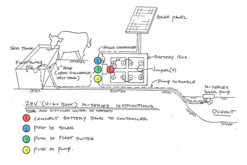
These systems can come in a variety of battery bank voltages. This is a 24v (4-6v battery) example. Can also come in 12v (2-6v), 12v (2-12v), 24v (2-12v), 36v (3-12v) 48v (4-12v).
