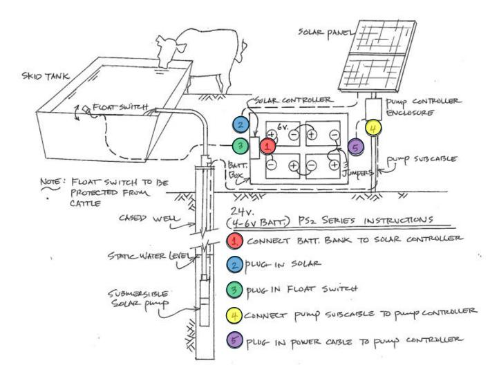
These systems can come in a variety of battery bank voltages. This is a 24v (4-6v battery) example. Can also come in 12v (2-6v), 12v (2-12v), 24v (2-12v), 36v (3-12v) 48v (4-12v).
